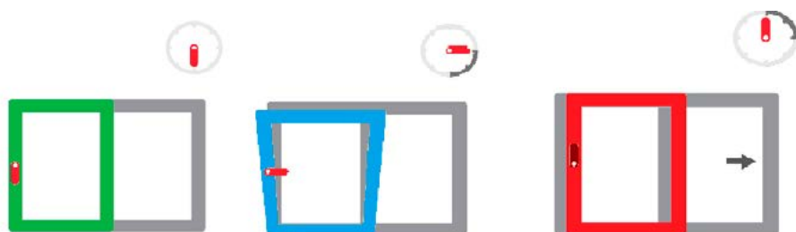
Drawing 4.2. Opening the Roto Patio Alversa KS tilt and slide door
