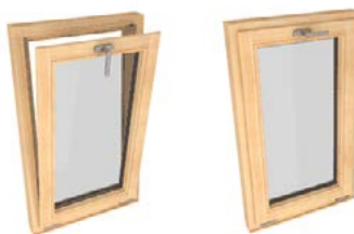
Figure 2.5. Inward opening window with a tilt only (bottom hung) sash
